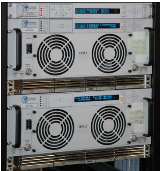
◀ 400W C-Band (4RU) 1:1 Phase Combined System
